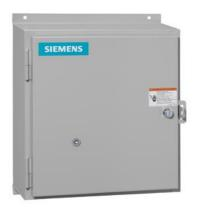
Reversing motor starter, Size 2 1/2, Three phase full voltage, Solid-state overload relay, OLR amp range 25-100A, Non-combination type, Enclosure type 4X fiberglass, Water/dust tight noncorrosive, Standard width enclosure
