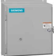
Reversing motor starter, Size 2 1/2, Three phase full voltage, Solid-state overload relay, OLR amp range 25-100A, 110V 50Hz / 120V 60Hz coil, Non-combination type, Enclosure type 4X fiberglass, Water/dust tight noncorrosive, Standard width enclosure
