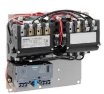
Reversing motor starter Size 2 1/2 Three phase full voltage Solid-state overload relay OLRelay amp range 25-100A 380-440/440-480V 50/60HZ coil Non-combination type Enclosure type (open)
