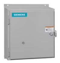
Reversing motor starter, Size 2 1/2, Three phase full voltage, Amb. compensate bimetal OLR, Contactor amp rating 60A, 110V 50Hz / 120V 60Hz coil, Noncombination type, Enclosure type 12, Dust/drip proof for indoors
