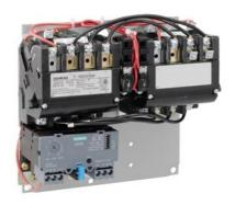
Reversing motor starter Size 1 3/4 Three phase full voltage Solid-state overload relay OLRelay amp range 10-40a 208VAC 60HZ coil Non-combination type Enclosure type (open)
