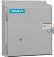
Reversing motor starter, Size 1, Three phase full voltage, Solid-state overload relay, OLR amp range 3-12A, Non-combination type, Enclosure type 4X fiberglass, Water/dust tight noncorrosive, Standard width enclosure
