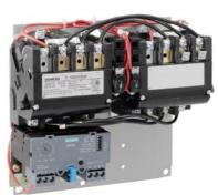
Reversing motor starter Size 1 Three phase full voltage Solid-state overload relay OLRelay amp range 0.25-1A 24VAC 50-60HZ coil Non-combination type Enclosure type (open)
