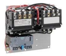
Reversing motor starter Size 1 Three phase full voltage Solid-state overload relay OLRelay amp range 0.25-1A 190-220/220-240V 50/60HZ coil Non-combination type Enclosure type (open)
