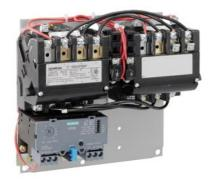
Reversing motor starter Size 0 Three phase full voltage Solid-state overload relay OLRelay amp range 5.5-22A 208VAC 60HZ coil Non-combination type Enclosure type (open)
