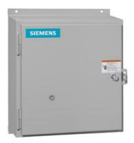
Reversing motor starter, Size 0, Three phase full voltage, Solid-state overload relay, OLR amp range 0.25-1A, Non-combination type, Enclosure type 4X fiberglass, Water/dust tight noncorrosive, Standard width enclosure
