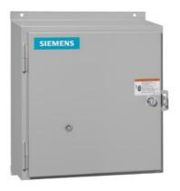
Reversing motor starter, Size 0, Three phase full voltage, Solid-state overload relay, OLR amp range 0.25-1A, 208VAC 60Hz coil, Non-combination type, Enclosure type 4X fiberglass, Water/dust tight noncorrosive, Standard width enclosure
