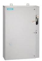
Non-reversing motor starter, Size 4, Three phase full voltage, Solid-state overload relay, OLR amp range 50-200A, 110V 50Hz / 120V 60Hz coil, Combination type, 150A circuit breaker, Encl NEMA type 4X 304 S-Steel, Water/dust tight noncorrosive, Standard width enclosure
