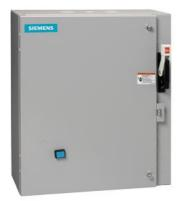
Non-reversing motor starter, Size 3, Three phase full voltage, Solid-state overload relay, OLR amp range 25-100A, Combination type, 125A circuit breaker, Enclosure NEMA type 1, Indoor general purpose use, Standard width enclosure
