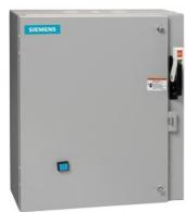
Non-reversing motor starter, Size 3, Three phase full voltage, Solid-state overload relay, OLR amp range 25-100A, Combination type, 125A circuit breaker, Enclosure NEMA type 1, Indoor general purpose use, Standard width enclosure
