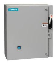
Non-reversing motor starter Size 3 Three phase full voltage Solid-state overload relay OLRelay amp range 25-100A 110-120/220-240VAC 60HZ coil Combination type 125Amp circuit breaker Enclosure NEMA type 1 Indoor general purpose use Standard width enclosure
