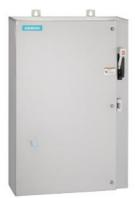
Non-reversing motor starter, Size 3, Three phase full voltage, Solid-state overload relay, OLR amp range 25-100A, Combination type, 125A circuit breaker, Encl NEMA type 4X 304 S-Steel, Water/dust tight noncorrosive, Extra-wide enclosure
