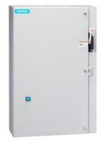
Non-reversing motor starter, Size 3, Three phase full voltage, Solid-state overload relay, OLR amp range 25-100A, 240V 50Hz / 277V 60Hz coil, Combination type, 125A circuit breaker, Enclosure NEMA type 1, Indoor general purpose use, Extrawide enclosure
