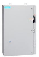
Non-reversing motor starter, Size 2 1/2, Three phase full voltage, Solid-state overload relay, OLR amp range 25-100A, Combination type, 100A circuit breaker, Encl NEMA type 4X 316 S-Steel, Water/dust tight noncorrosive, Standard width enclosure
