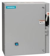
Non-reversing motor starter Size 2 1/2 Three phase full voltage Solid-state overload relay OLRelay amp range 25-100A 208VAC 60HZ coil Combination type 100A circuit breaker Enclosure NEMA type 1 Indoor general purpose use Standard width enclosure
