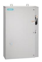
Non-reversing motor starter, Size 2 1/2, Three phase full voltage, Solid-state overload relay, OLR amp range 25-100A, 240V 50Hz / 277V 60Hz coil, Combination type, 100A circuit breaker, Encl NEMA type 4X 304 S-Steel, Water/dust tight noncorrosive, Extra-wide enclosure
