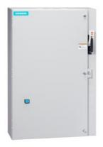
Non-reversing motor starter, Size 2 1/2, Three phase full voltage, Solid-state overload relay, OLR amp range 25-100A, 110V 50Hz / 120V 60Hz coil, Combination type, 100A circuit breaker, Enclosure NEMA type 1, Indoor general purpose use, Extra-wide enclosure
