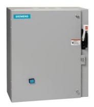
Non-reversing motor starter, Size 1, Three phase full voltage, Solid-state overload relay, OLR amp range 5.5-22A, Combination type, 25A circuit breaker, Enclosure NEMA type 1, Indoor general purpose use, Extra-wide enclosure
