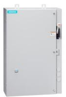
Non-reversing motor starter, Size 1, Three phase full voltage, Solid-state overload relay, OLR amp range 0.75-3.4A, 110V 50Hz / 120V 60Hz coil, Combination type, 3A circuit breaker, Enclosure NEMA type 4/12, Water/dust tight for outdoors, Extrawide enclosure
