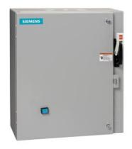
Non-reversing motor starter, Size 0, Three phase full voltage, Solid-state overload relay, OLR amp range 3-12A, 240V 50Hz / 277V 60Hz coil, Combination type, 10A circuit breaker, Enclosure NEMA type 1, Indoor general purpose use, Extra-wide enclosure
