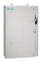
Non-reversing motor starter, Size 4, Three phase full voltage, Solid-state overload relay, OLR amp range 50-200A, Combination type, 200A non-fusible disconnect, Encl NEMA type 4X 304 S-Steel, Water/dust tight noncorrosive, Standard width enclosure
