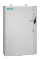
Non-reversing motor starter Size 4 Three phase full voltage Solid-state overload relay OLRelay amp range 50-200A 550/575-600 50/60HZ coil Combination type 200A fusible disconnect 200A/600V fuse clip Encl NEMA type 4X 304 S-steel Water/dust tight noncorrosive Standard width enclosure
