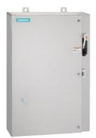
Non-reversing motor starter, Size 4, Three phase full voltage, Solid-state overload relay, OLRelay amp range 50-200A, 550/575 600 50/60HZ coil, Combination type, 200A non-fusible disconnect, Encl NEMA type 4X 304 S-steel Water/dust tight noncorrosive, Standard width enclosure
