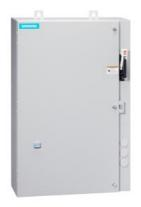
Non-reversing motor starter, Size 4, Three phase full voltage, Solid-state overload relay, OLR amp range 50-200A, 110V 50Hz / 120V 60Hz coil, Combination type, 200A fusible disconnect, 200A/250V fuse clip, Enclosure NEMA type 4/12, Water/dust tight for outdoors, Standard width enclosure
