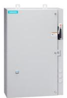
Non-reversing motor starter, Size 4, Three phase full voltage, Solid-state overload relay, OLR amp range 50-200A, 208VAC 60Hz coil, Combination type, 200A fusible disconnect, 200A/600V fuse clip, Enclosure NEMA type 4/12, Water/dust tight for outdoors, Standard width enclosure
