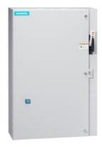
Non-reversing motor starter Size 4 Three phase full voltage Solid-state overload relay OLRelay amp range 50-200A 550/575-600 50/60HZ coil Combination type 200A fusible disconnect 200A/600V fuse clip Enclosure NEMA type 1 Indoor general purpose use Standard width enclosure
