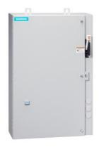
Non-reversing motor starter, Size 3, Three phase full voltage, Solid-state overload relay, OLR amp range 25-100A, Combination type, 100A fusible disconnect, 100A/250V fuse clip, Encl NEMA type 4X 304 S-Steel, Water/dust tight noncorrosive, Standard width enclosure
