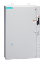
Non-reversing motor starter, Size 3, Three phase full voltage, Solid-state overload relay, OLR amp range 25-100A, Combination type, 100A fusible disconnect, 100A/250V fuse clip, Enclosure NEMA type 4/12, Water/dust tight for outdoors, Standard width enclosure
