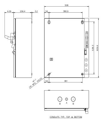
CONDUIT SIZE Ø12.7 & Ø19 CONDUIT Ø31.8 & Ø38.1 CONDUIT
