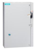
Non-reversing motor starter, Size 3, Three phase full voltage, Solid-state overload relay, OLR amp range 25-100A, 110V 50Hz / 120V 60Hz coil, Combination type, 200A fusible disconnect, 200A/250V fuse clip, Enclosure NEMA type 1, Indoor general purpose use, Standard width enclosure
