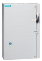
Non-reversing motor starter, Size 3, Three phase full voltage, Solid-state overload relay, OLR amp range 25-100A, Combination type, 200A fusible disconnect, 200A/250V fuse clip, Enclosure NEMA type 1, Indoor general purpose use, Standard width enclosure
