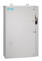
Non-reversing motor starter, Size 3, Three phase full voltage, Solid-state overload relay, OLR amp range 25-100A, 208VAC 60Hz coil, Combination type, 100A nonfusible disconnect, Encl NEMA type 4X 304 S-Steel, Water/dust tight noncorrosive, Extra-wide enclosure
