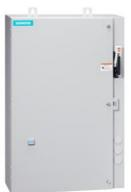
Non-reversing motor starter, Size 3, Three phase full voltage, Solid-state overload relay, OLR amp range 25-100A, 208VAC 60Hz coil, Combination type, 100A fusible disconnect, 100A/600V fuse clip, Enclosure NEMA type 4/12, Water/dust tight for outdoors, Extra-wide enclosure
