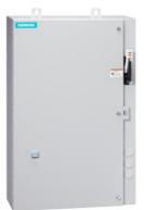
Non-reversing motor starter, Size 2 1/2, Three phase full voltage, Solid-state overload relay, OLR amp range 25-100A, 24VDC coil, Combination type, 100A fusible disconnect, 100A/600V fuse clip, Encl NEMA type 4X 304 S-Steel, Water/dust tight noncorrosive, Standard width enclosure
