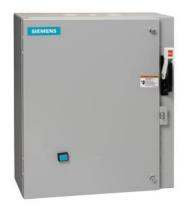
Non-reversing motor starter, Size 2 1/2, Three phase full voltage, Solid-state overload relay, OLR amp range 25-100A, Combination type, 100A non-fusible disconnect, Enclosure NEMA type 1, Indoor general purpose use, Standard width enclosure
