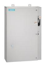
Non-reversing motor starter, Size 2 1/2, Three phase full voltage, Solid-state overload relay, OLR amp range 25-100A, 208VAC 60Hz coil, Combination type, 60A fusible disconnect, 60A/600V fuse clip, Encl NEMA type 4X 304 S-Steel, Water/dust tight noncorrosive, Extra-wide enclosure
