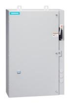
Non-reversing motor starter, Size 2 1/2, Three phase full voltage, Solid-state overload relay, OLR amp range 25-100A, Combination type, 100A non-fusible disconnect, Enclosure NEMA type 4/12, Water/dust tight for outdoors, Extra-wide enclosure
