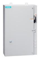
Non-reversing motor starter, Size 2 1/2, Three phase full voltage, Solid-state overload relay, OLR amp range 25-100A, 110V 50Hz / 120V 60Hz coil, Combination type, 60A fusible disconnect, 60A/600V fuse clip, Enclosure NEMA type 4/12, Water/dust tight for outdoors, Extra-wide enclosure
