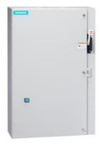
Non-reversing motor starter, Size 2 1/2, Three phase full voltage, Solid-state overload relay, OLR amp range 25-100A, 110V 50Hz / 120V 60Hz coil, Combination type, 60A fusible disconnect, 60A/600V fuse clip, Enclosure NEMA type 1, Indoor general purpose use, Extra-wide enclosure
