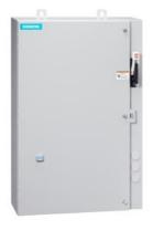
Non-reversing motor starter, Size 2, Three phase full voltage, Solid-state overload relay, OLR amp range 13-52A, 240V 50Hz / 277V 60Hz coil, Combination type, 60A non-fusible disconnect, Encl NEMA type 4X 304 S-Steel, Water/dust tight noncorrosive, Extra-wide enclosure
