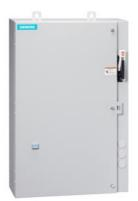
Non-reversing motor starter, Size 1 3/4, Three phase full voltage, Solid-state overload relay, OLR amp range 10-40A, 24VDC coil, Combination type, 60A non-fusible disconnect, Enclosure NEMA type 4/12, Water/dust tight for outdoors, Extra-wide enclosure
