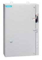
Non-reversing motor starter, Size 1 3/4, Three phase full voltage, Solid-state overload relay, OLR amp range 10-40A, 24VAC 50-60Hz coil, Combination type, 60A fusible disconnect, 60A/250V fuse clip, Enclosure NEMA type 4/12, Water/dust tight for outdoors, Extra-wide enclosure
