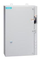
Non-reversing motor starter, Size 1 3/4, Three phase full voltage, Solid-state overload relay, OLR amp range 10-40A, 208VAC 60Hz coil, Combination type, 60A non-fusible disconnect, Enclosure NEMA type 4/12, Water/dust tight for outdoors, Extra-wide enclosure
