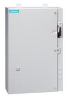
Non-reversing motor starter, Size 1, Three phase full voltage, Solid-state overload relay, OLR amp range 10-40A, Combination type, 60A non-fusible disconnect, Encl NEMA type 4X 304 S-Steel, Water/dust tight noncorrosive, Extra-wide enclosure
