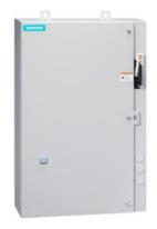
Non-reversing motor starter, Size 1, Three phase full voltage, Solid-state overload relay, OLR amp range 5.5-22A, 110V 50Hz / 120V 60Hz coil, Combination type, 30A fusible disconnect, 30A/250V fuse clip, Enclosure NEMA type 4/12, Water/dust tight for outdoors, Extra-wide enclosure
