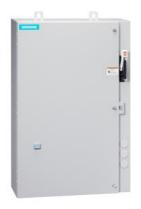
Non-reversing motor starter, Size 1, Three phase full voltage, Solid-state overload relay, OLR amp range 5.5-22A, Combination type, 30A fusible disconnect, 30A/250V fuse clip, Enclosure NEMA type 4/12, Water/dust tight for outdoors, Extra-wide enclosure
